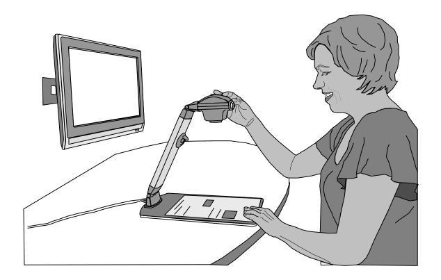
Place the material you wish to read on the reading table, looking at the TV screen to see where you are. Adjust the magnification to suit. Ensure the camera head is horizontal for optimum image quality.
