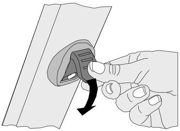
The light can be rotated as shown. It should be adjusted so that it shines on an area centred about the camera's image.
